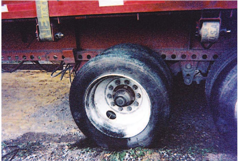
**TIRE DAMAGE:** Tires show damage caused by electrical contact. Eight of the truck's tires were ruined by the contact. This accident could have been much worse than it was.
