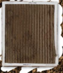
Dirty air filters cause a heating and cooling system to work harder and break down faster. That's because unfiltered dust and grime works into critical parts, creating friction that causes unnecessary wear and, eventually, failure.
