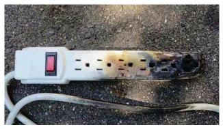
**HEATER SAFETY:** Do not plug heaters into power strips or extension cords as they are not able to handle the extra current a heater requires.
